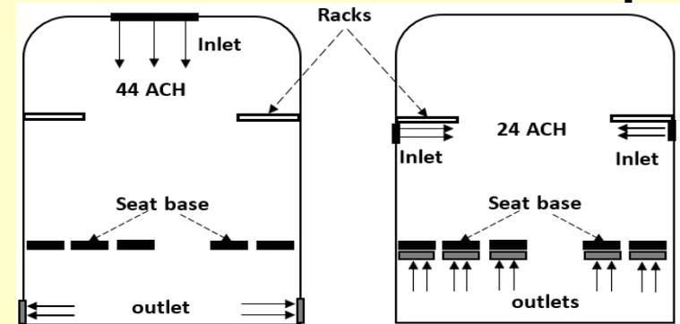
Two typical ventilation configurations
